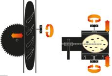
2. Possibility of adjusting the blade to the thickness of the baguette and to the desired slice.
