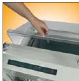
When closed, the optional safety lid triggers start-up. It opens automatically when slicing is complete.
